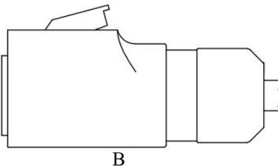
Plug the B-end of the emergency cable (as shown on the left) into the socket on the foot control panel.
