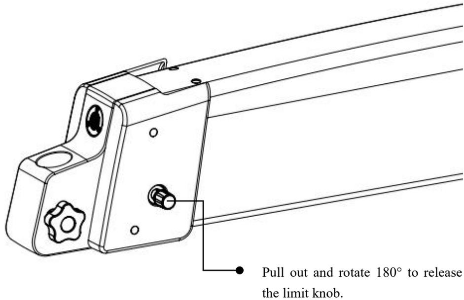
2. Check joint brakes of support arm and suspension arm
