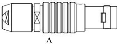
Plug the A-end of the emergency cable (as shown on the left) into the socket on the XY coupling.
