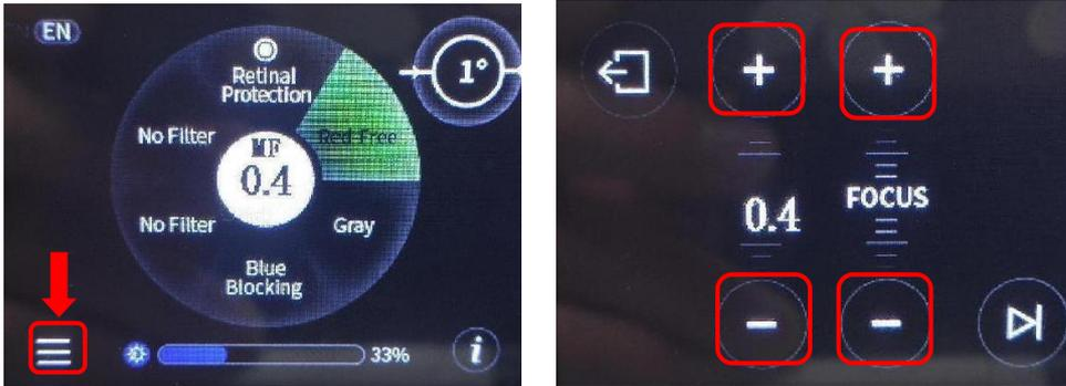
3. Adjusting the movement of the XY coupling: Tap the
