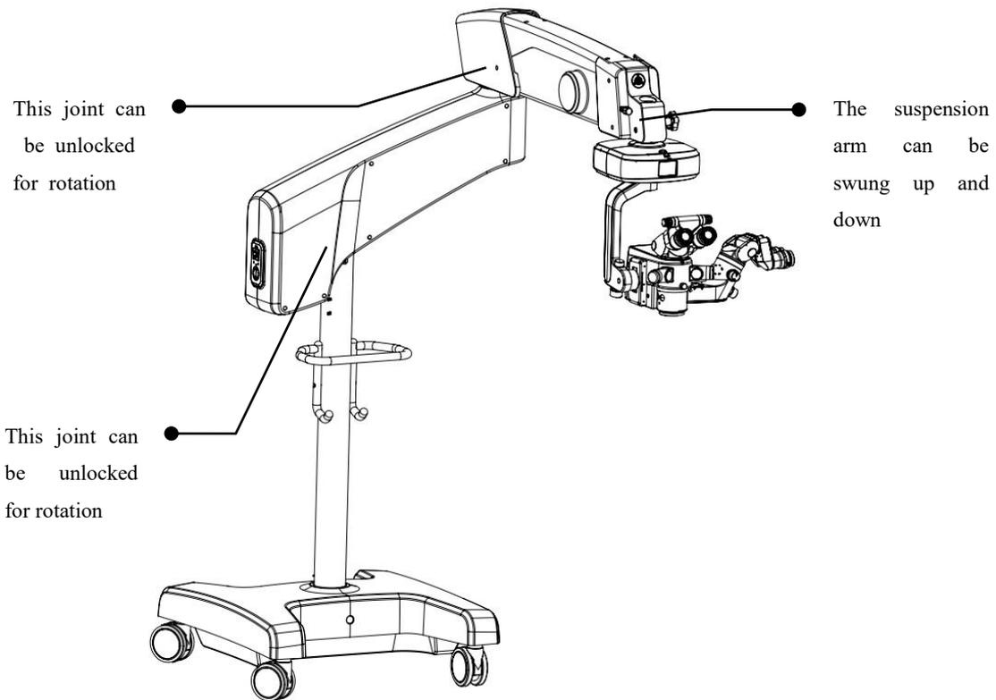
3. Adjust the microscope part to rotate and swing
