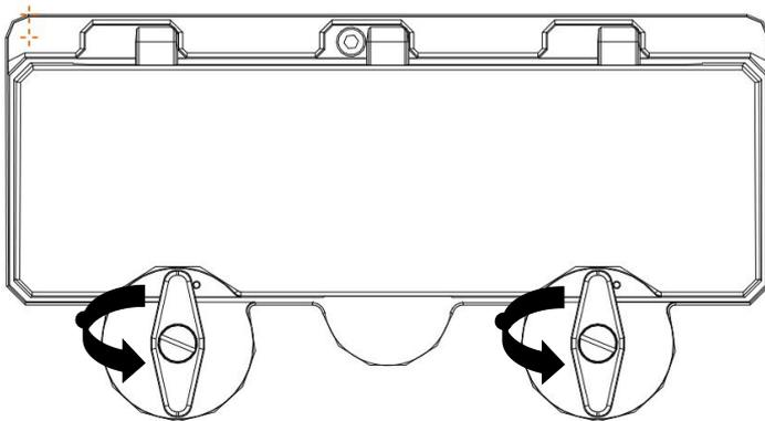
Open the battery cover to remove the battery, replace with a new battery (pay attention to the positive and negative poles of the battery), then close the battery cover with the screws and lock it.
