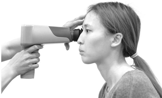
Step 3: Carefully move the device back and forth until the whole fundus is displayed on the screen.
