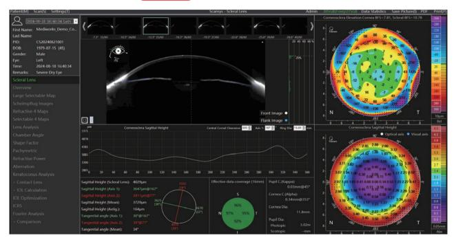
Scansys can capture 60 high-definition Scheimpflug images of corneosclera in a single scan, covering a 16mm-diameter of corneoscleral area. It can display the corneoscleral sagittal height in a 360° panoramic view without any multiple scans and image stitching, and provide 13 key parameters so as to offer comprehensive and accurate data support for scleral lens fitting.
